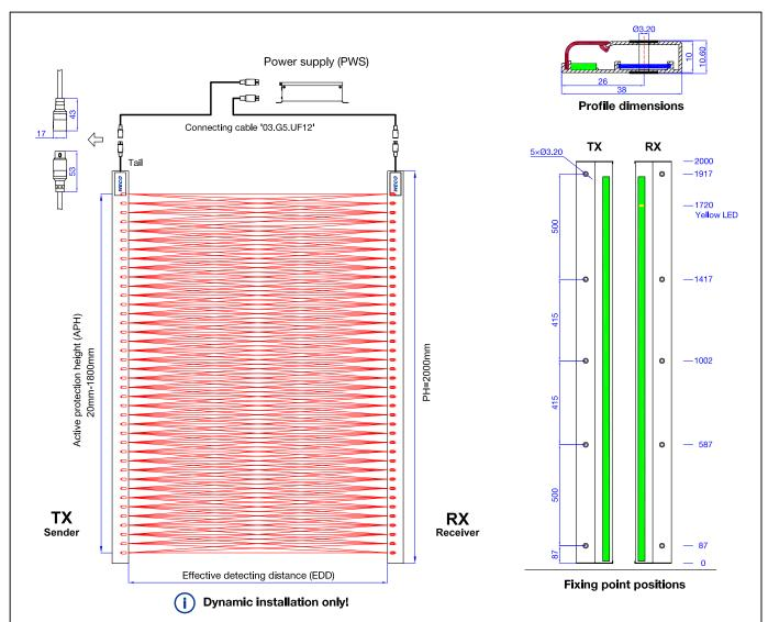
**Note:** A fuzzy algorithm is taken to calculate the position of doors, which only functions in dynamic installation and adjusts distances and times based on the speed of the door operating system. The information below is for general guidance.
